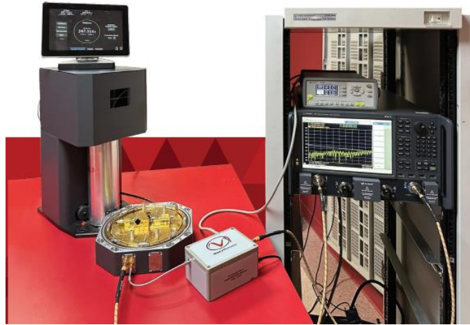
Figure 4: Full system setup with the Cryostation® s200 and the CT-Series Cryogenic Automated Tuner
