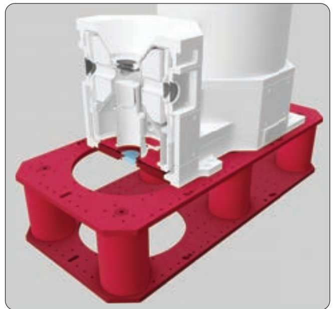
OptiCool cryostat equipped with bottom window mounted on top of the riser platform.
