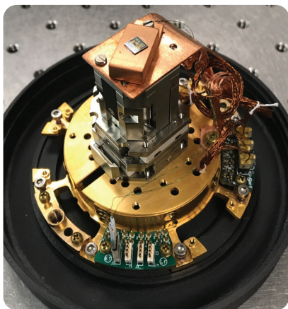
Pod shown with one X300 standard wiring bay and one X301 attocube wiring bay. Thermal and electrical connections between the pod and cryostat are made by simply plugging in the pod.
