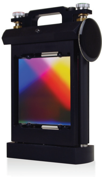
The Kymera's dual-grating turret, shown here, can be easily removed and replaced with optional gratings to achieve the required spectral bandwidth or resolution required. Integrated RFID tags allow for easy identification of a grating in the MultiVu software.
