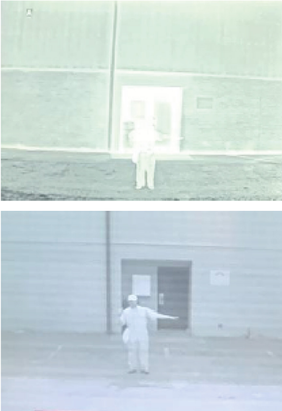
Figure 4: Current thermal DVE (Above). SWIR DVE (Below). You can see the difference in clarity between the two images. **
