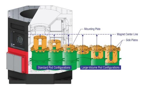
The location of the mounting plate relative to the Magnet Center Line can be adjusted by swapping out the two curved Side Plates. There are three standard sizes of side plates that come with either the standard or large-volume sample pod. These side plates allow the mounting plate to be positioned at three different distances either above or below the pod flange (see illustration above).
