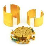
The Standard Sample Pod allows you to position the mounting plate at three different locations within the sample volume. This is accomplished by swapping out the pod side plates. The available side plates allow you to locate the mounting plate at either 12.4 mm, 32.8 mm, or 56.4 mm below the magnet center line position. The standard sample pod is useful for mounting smaller experimental setups, shorter stacks of positioners, or samples higher up in the sample volume.
