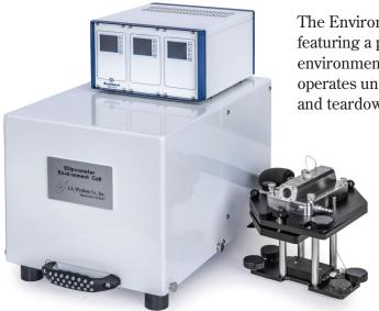
The Environment Cell is an optional accessory for the M-2000 and RC2 featuring a patented vapor-delivery system to create relative pressure environments using a wide variety of solvents. The Environment Cell operates under standard atmospheric conditions enabling quick setup and teardown of experiments.
