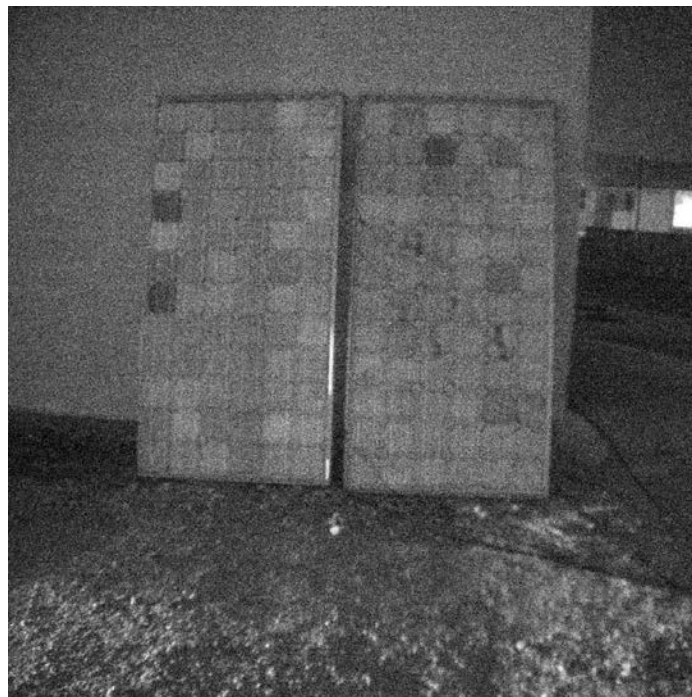
Figure 7: Falcon, NIR video of the same solar panels with variable currents at 20 fps. Again the defective cells are clearly visible. Contrast could be improved using a visible filter.
