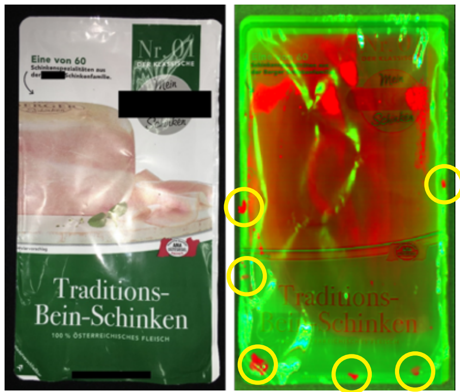
Inspection result with SPECIM FX17, contaminations in the seal marked with a yellow circle
