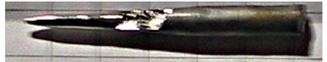
Fig. 3. Single crystal of \text{CeRh}_3\text{Si}_2 grown by the Czochralski technique in the tetra-arc furnace installed in Wrocław.
