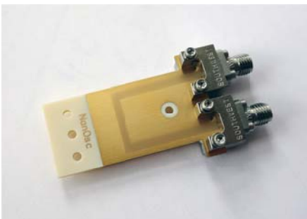
Coplanar Waveguide (CPW) for room temperature PhaseFMR
