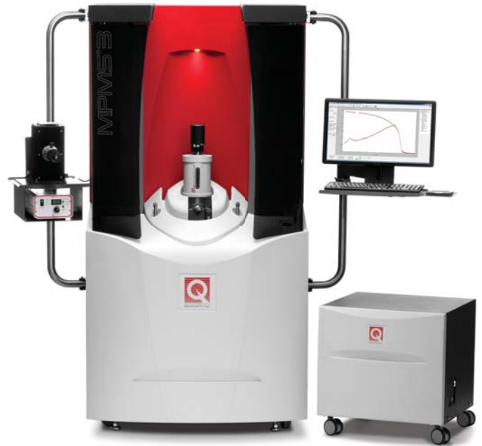
MPMS 3 shown with Quantum Design light source and controller for FOSH.
