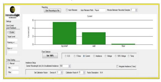
BAR - Allows multisystem, datalogging and displays the user switchable parameter in a bar graph. The expandable graph can accommodate up to 32 systems simultaneously with use of hub(s). User can enter nicknames for each unit to define the location, application, version, serial number, etc. Customer can program max and min warning levels and use color coded bar responses for easy troubleshooting.
