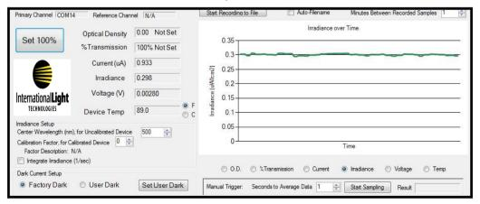
**TREND** - Records all 6 parameters while displaying the trend over time for the user switchable parameter. Multiple examples of trend can be run simultaneously to allow multi-unit comparisons. Trend also has a user-friendly calibration feature.
