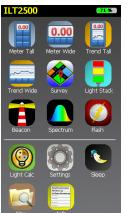
**Survey** allows data to be sorted by location or light source and **Light Stack** has a programmable color changing display (red/yellow/ green) and sound alert for quick troubleshooting.
