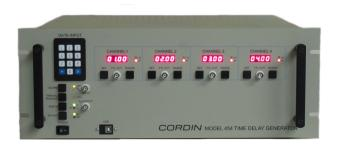
The Cordin Model 454 Time Delay Generator is a very reliable and robust delay unit. It will produce four channels of delayed output with delay ranges from 10 nanoseconds to 99.99 milliseconds. Delay values have a four digit resolution. The full range of delays is covered by four range settings; 00.00 milliseconds, 0.000 milliseconds, 00.00 microseconds and 0.000 microseconds. Pulse width of the output is selectable between 1.0 microseconds and 100 microseconds.
