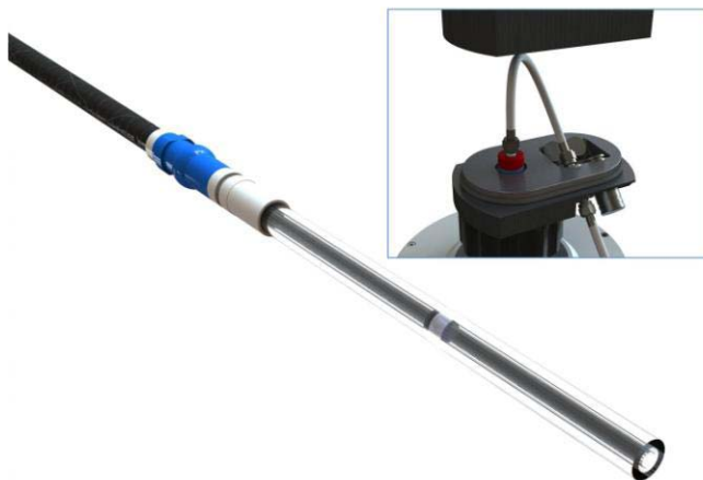
Fig. 5. Improved FOSH sample holder design where the bottom loading spring is moved to the top of the sample holder in order to reduce background signal thus further improve moment resolution.
