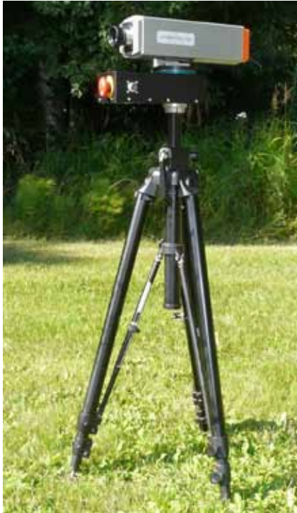
Rotating Scanner mounted on a cased Spectral Camera on top of a standard tripod
