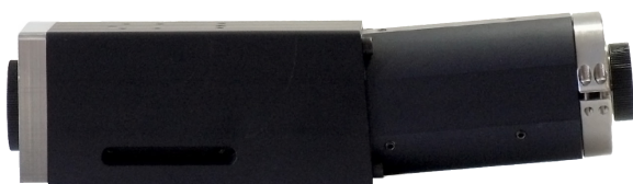
ImSpector N17E spectrograph, side view
