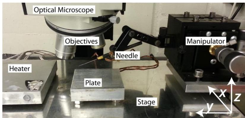
Figure 2: A nanowire transferring setup from TU Delft
