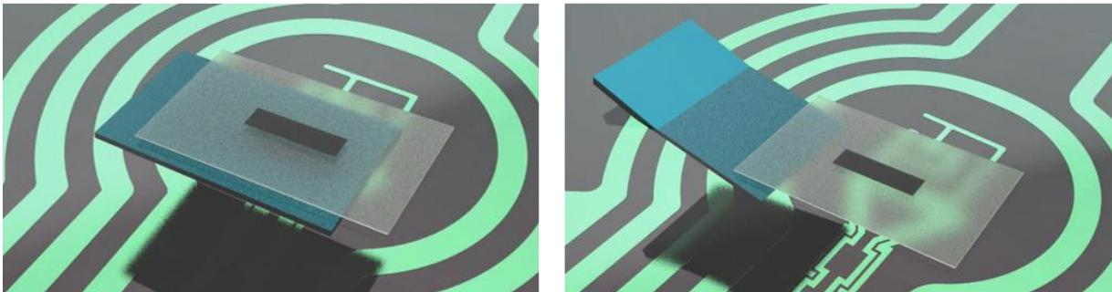
4. In the same beaker where graphene and the polymer is peeled off, use the micromanipulator to carefully move graphene to our Nano-Chip
