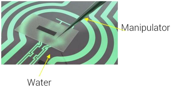
5. Align graphene with Nano-Chip as good as possible, and then drain the water to bring graphene and Nano-Chip in contact.
