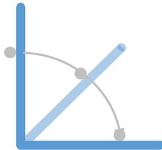
Figure 3: Typical trajectory to pick up a nanowire. Grey spot indicates the needle and the nanowires are represented here as blue lines. In reality, nanowires will bend during picking up process.
