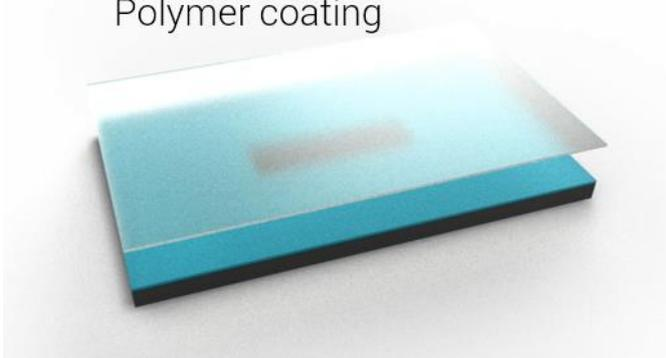
3. Then dip the polymer coated substrate in water. Due to the hydrophobic force, graphene will be peeled off from the substrate together with the polymer layer.
