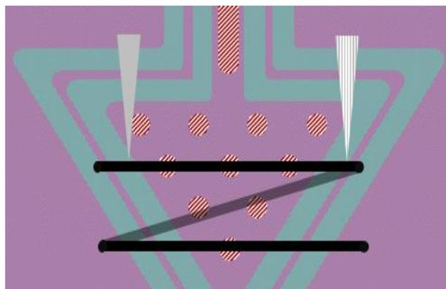
Figure 4: Moving of nanowires on our Nano-Chip substrate. The nanowire (blackline) which does not land on the right spots could be push with the tip (grey triangle) to the right location.
