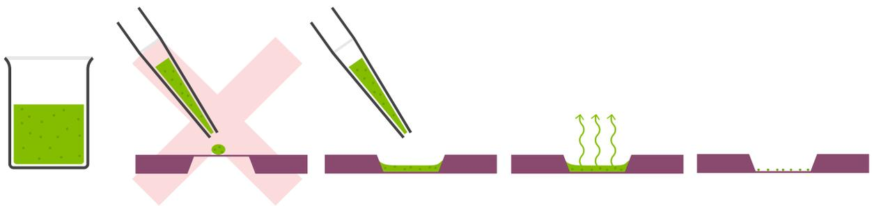
*Figure 1. Drop casting method.*
