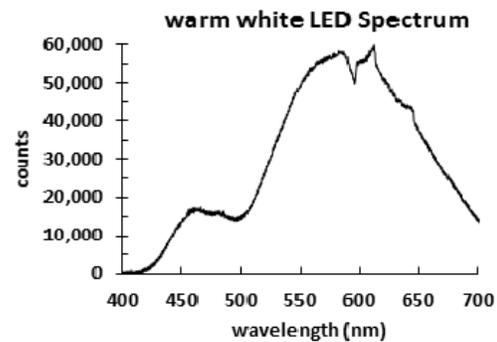
Figure 3(b). LED spectrum for  $f/6.45$  measurements.
