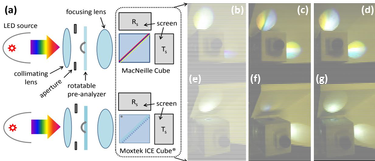
Figure 2. Low  $f/\#$  performance comparison between polarizing beam splitter cubes. Measurement schematic (a) and results for MacNeille cube (b-d) and Moxtek *ICE Cube* (e-g) showing blocking state (b, e), passing state (c, f), and beamsplitting (d, g) configurations. Notice the poor color shift when using a MacNeille cube (c-d).
