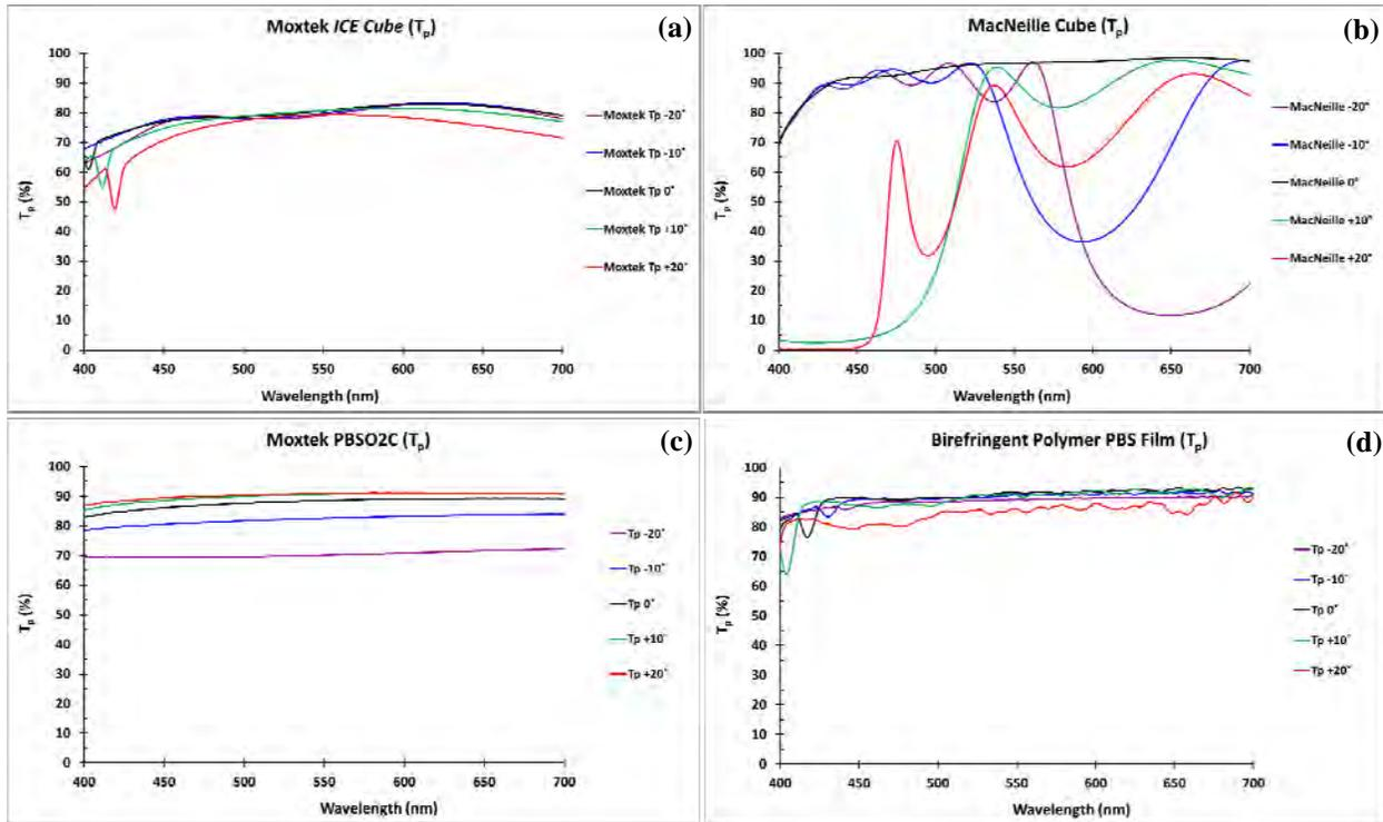
Figure 6. Variable angle passing state transmittance ( $T_p$ ) performance comparison for a typical Moxtek *ICE Cube* and PBS product and for competing beamsplitters for  $0^\circ$  to  $\pm 20^\circ$  azimuthal angle of incidence. (a) Moxtek *ICE Cube* performance. (b) MacNeille Cube performance. (c) Moxtek ProFlux PBS02C wire-grid PBS plate. (d) Birefringent Polymer PBS film.
