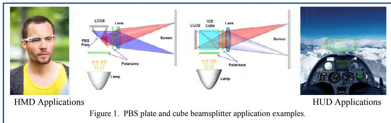
Figure 1. PBS plate and cube beamsplitter application examples.
