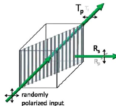
Figure 4. Moxtek *ICE Cube* beamsplitter schematic showing embedded wire grid polarizer as well as passing state transmittance ( $T_p$ ) and blocking state reflectance ( $R_s$ ). The weaker passing state reflectance ( $R_p$ ) and blocking state transmittance ( $T_s$ ) can be further removed using clean-up polarizers.
