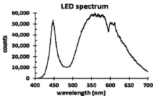
Figure 3(a). LED spectrum for  $f/1.74$  measurements.
