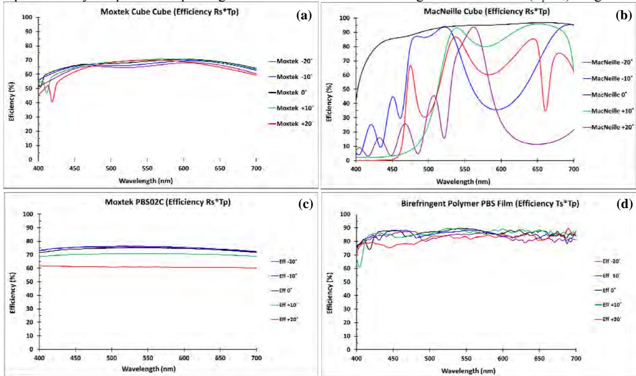
Figure 8. Variable angle efficiency ( $T_p \cdot R_s$ ) for a typical Moxtek *ICE Cube* and competing beamsplitter from 0° to ±20° azimuthal angles of incidence. (a) Moxtek *ICE Cube* performance. (b) MacNeille Cube performance. (c) Moxtek ProFlux PBS02C wire-grid PBS plate. (d) Birefringent Polymer PBS film.
