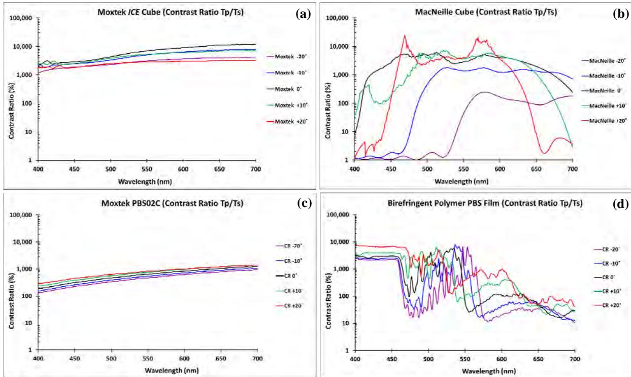
Figure 7. Variable angle contrast ratio ( $T_p/T_s$ ) performance for a typical Moxtek *ICE Cube* and competing beamsplitters for 0° to ±20° angle of incidence. (a) Moxtek *ICE Cube* performance. (b) MacNeille Cube performance. (c) Moxtek ProFlux PBS02C wire-grid PBS plate. (d) Birefringent Polymer PBS film.
