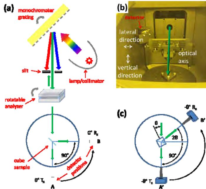
Figure 5. (a) Simplified measurement schematic in normal incidence ( $0^\circ$ ) configuration. (b) Inside view of Agilent Universal Measurement Accessory. (c) Measurement configuration for an azimuthal sample angle of  $-\theta^\circ$
