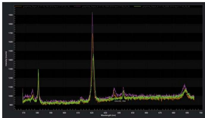
Raman spectra of graphene at 10K, 100K and 200K
