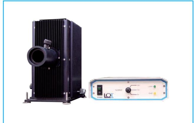
Some models have UV glass envelopes with a lower transmission between 167 - 250 nm. The 167 nm line (responsible for most of the produced ozone) is completely absorbed.
